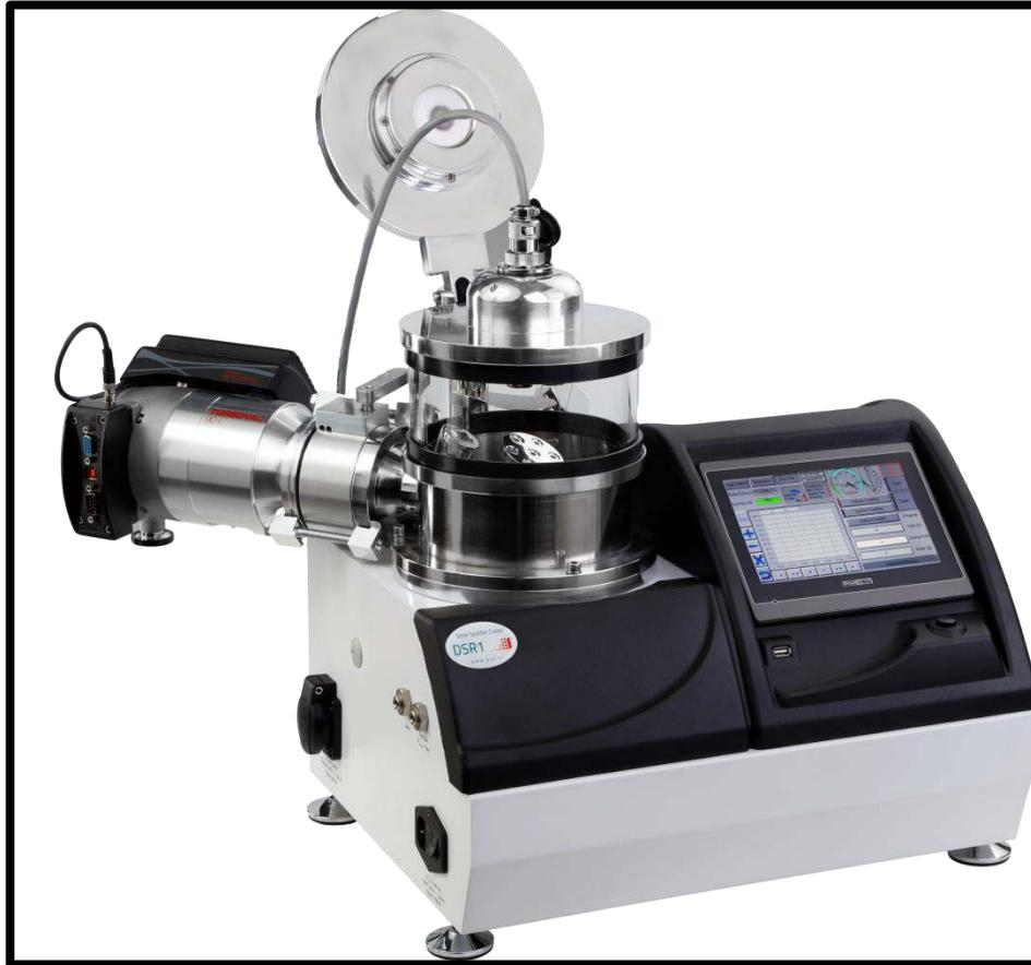
The DSCT is configured as a sputter coater and fiber carbon coater with interchangeable heads in one instrument suitable for Scanning Electron Microscope (SEM) sample preparation. A wide range of materials could be deposited by DSCT such as gold (Au), platinum / palladium (Pt / Pd) alloy, silver (Ag), chromium (Cr), tungsten (W), iridium (Ir) and etc.
