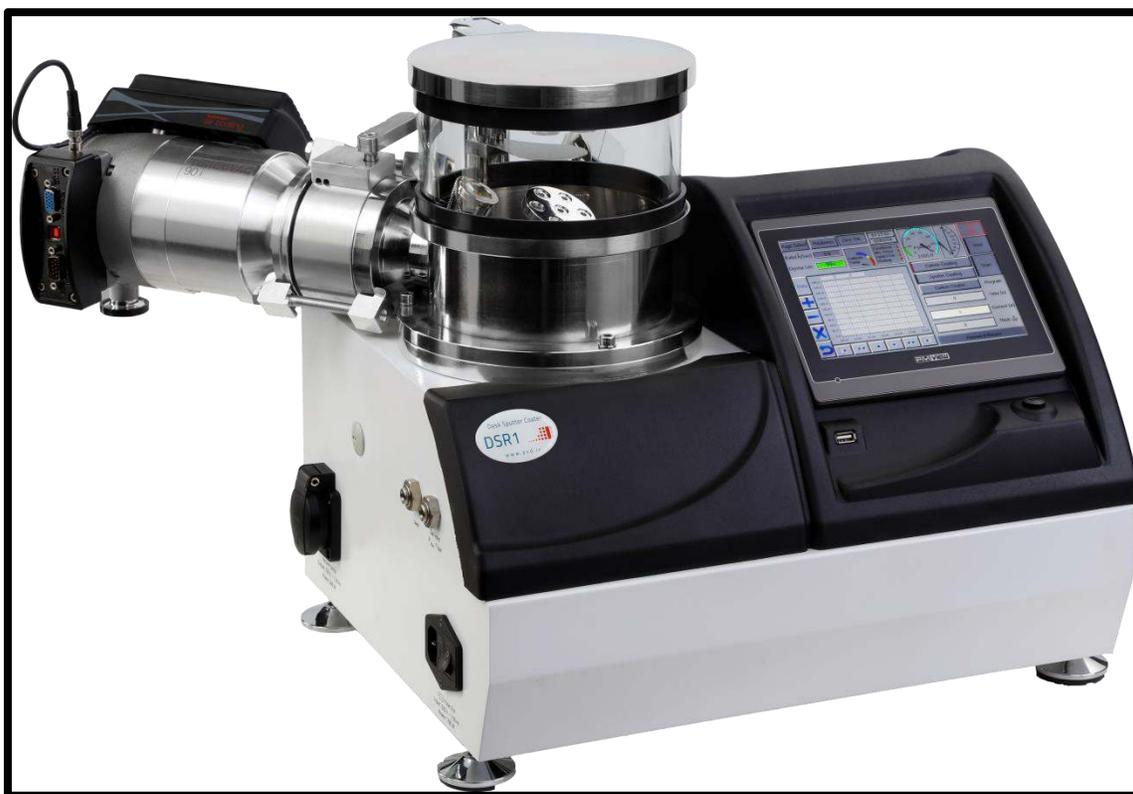
The DST1-170 is configured as a sputter coater suitable for Scanning Electron Microscope (SEM) sample preparation. A wide range of materials could be deposited by DST1-170 such as gold (Au), platinum/palladium (Pt/Pd) alloy, silver (Ag), chromium (Cr), tungsten (W), iridium (Ir) and etc.
