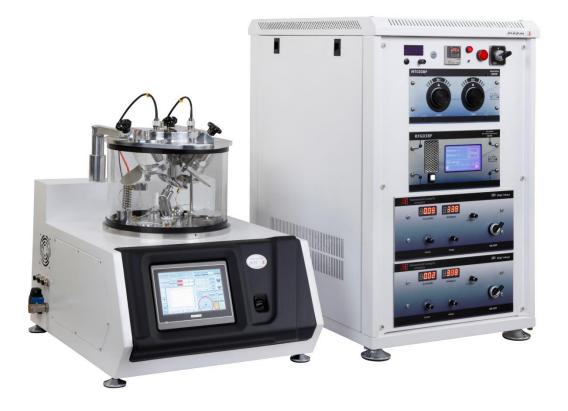
The DST3 is equipped with a large chamber (300 mm diameter) and three 2" diameter water cooled cathodes which make it suitable for long time deposition.
