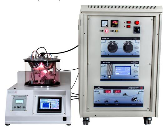
The DST3 is equipped with a large chamber and a water circulation cooling system for each cathodes which make it suitable for sputtering; a single large diameter specimen; and co-sputtering; a small diameter specimen.
